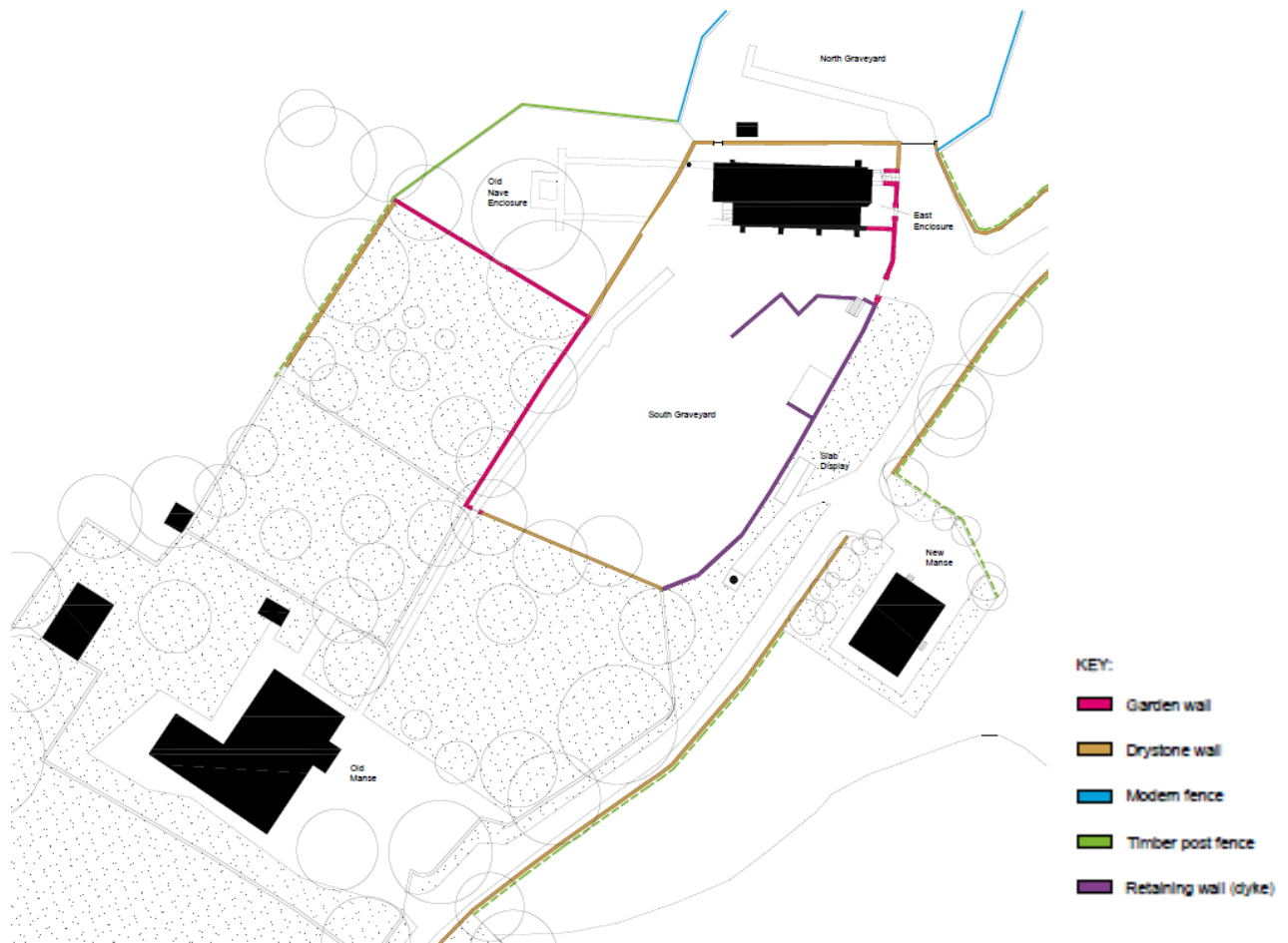
Fig 3: Site plan showing enclosure and boundary walls.
